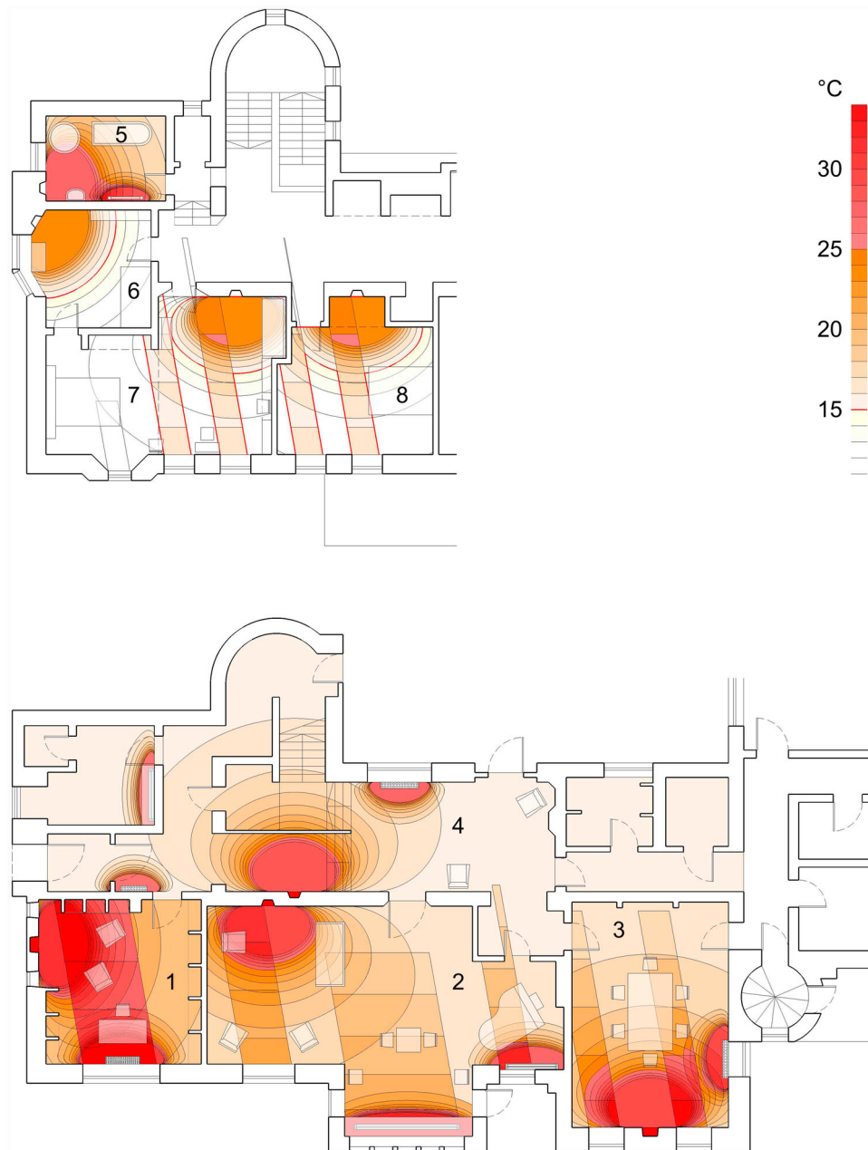
Figure 30. Floor plans with isotherms indicating operative temperature due to fireplaces, radiators and solar gains on the winter solstice. Key: 1. Library; 2. Drawing Room; 3. Dining Room; 4. Hallway; 5. Bathroom; 6. Dressing Room; 7. The White Bedroom; 8. Second Bedroom.
